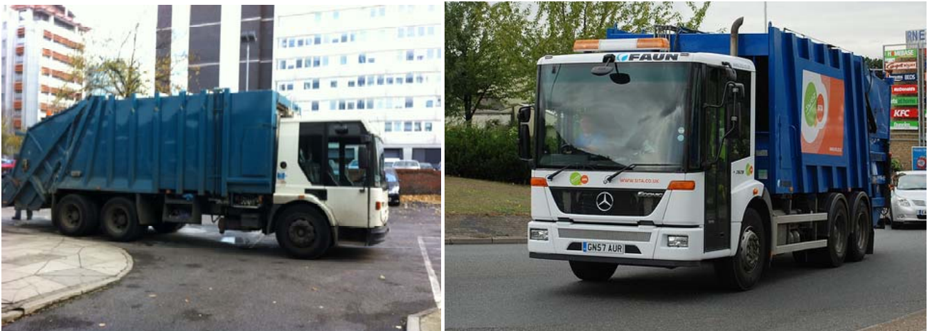
Fig 4.1 Refuse vehicles with and without sideguards
