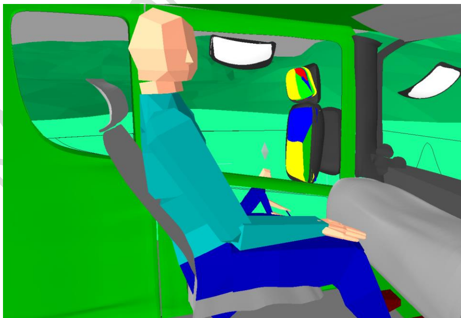
Figure 6. The view through the eyes of the driver. The benefit of the new lower door window is reduced when there is a passenger in the Cat. N3 vehicle.
